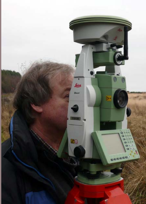
Leica TCRA1203 equipped with Smartstation GPS
